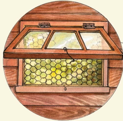
Window secured with chicken wire and a locking system
